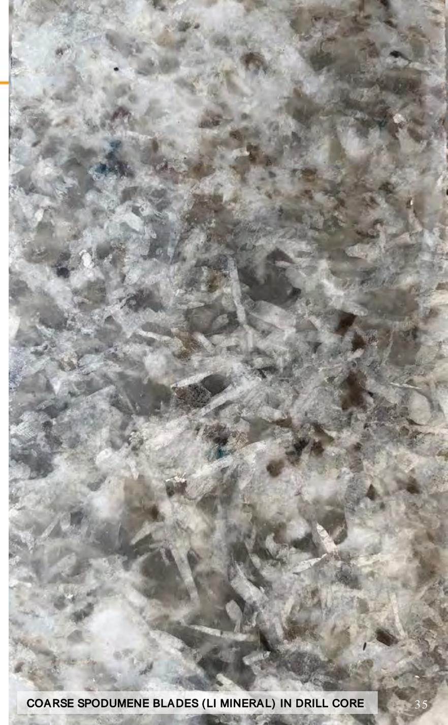
COARSE SPODUMENE BLADES (LI MINERAL) IN DRILL CORE
